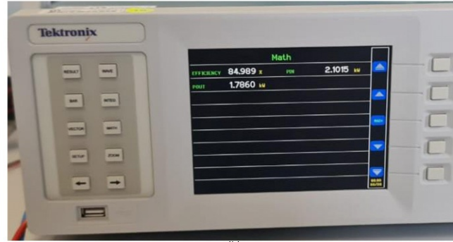
Fig. 8. Experimental results (a) Input 400 Hz voltage and current ( v_1 , i_1 ) and output dc side voltage and current ( v_{dc} and i_{dc} ) (b) the input and output power measured by the power analyzer.
